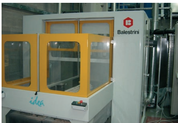
Photograph 1 CNC routing machine with interlocked doors
