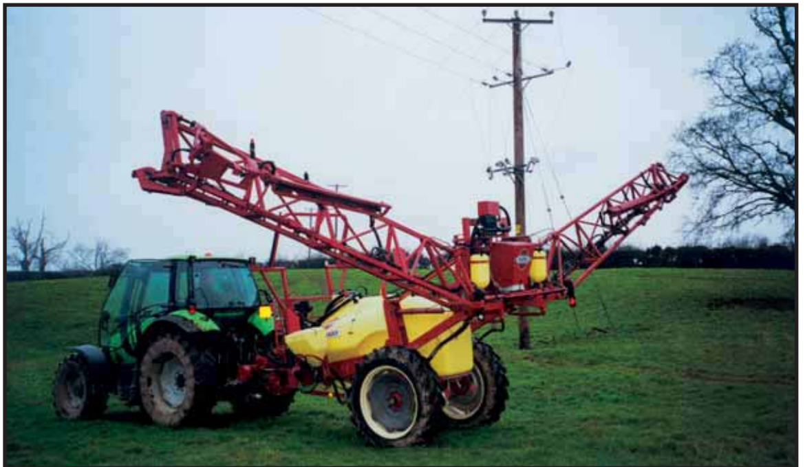
Consider using warning labels on high-reach equipment such as some crop sprayers
