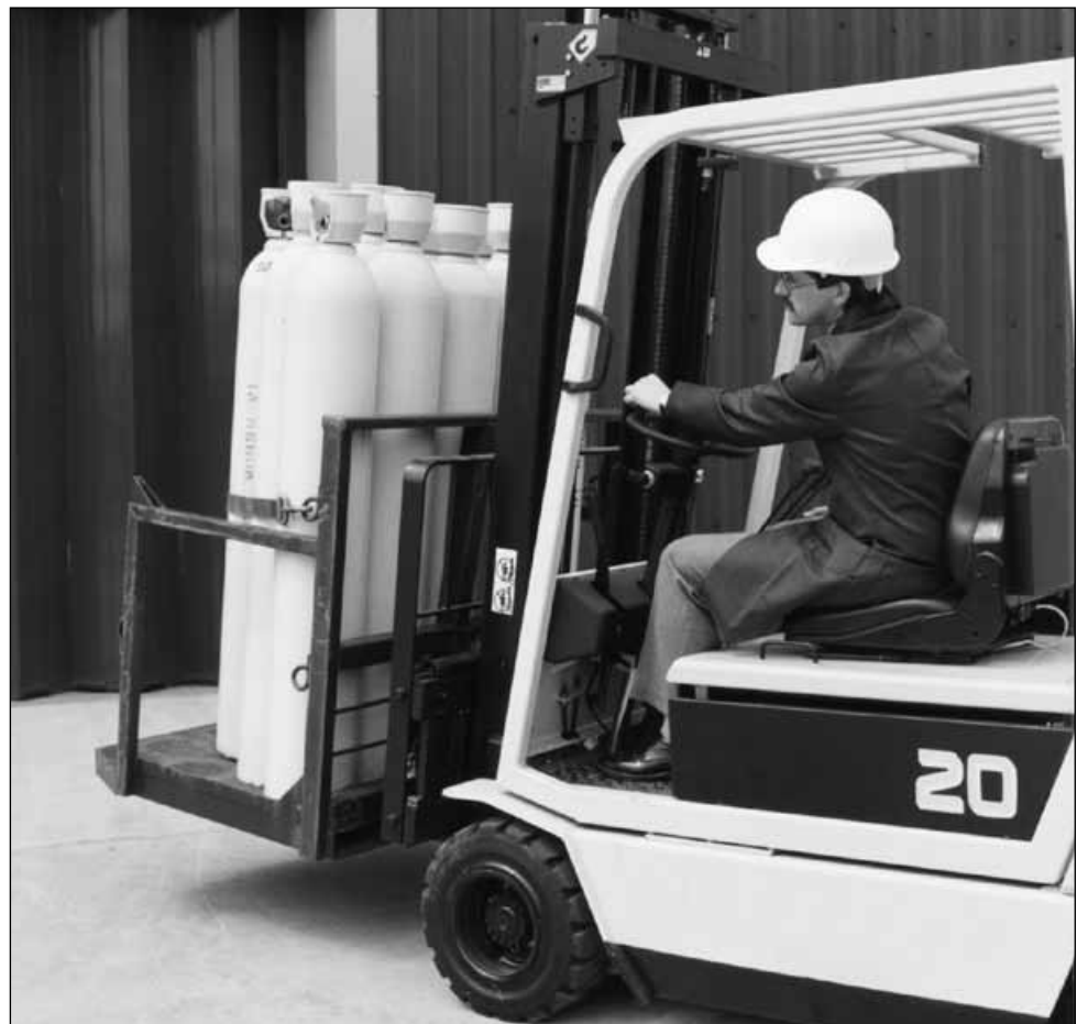
Figure 10 Cylinders on a carrying frame moved by fork-lift truck
