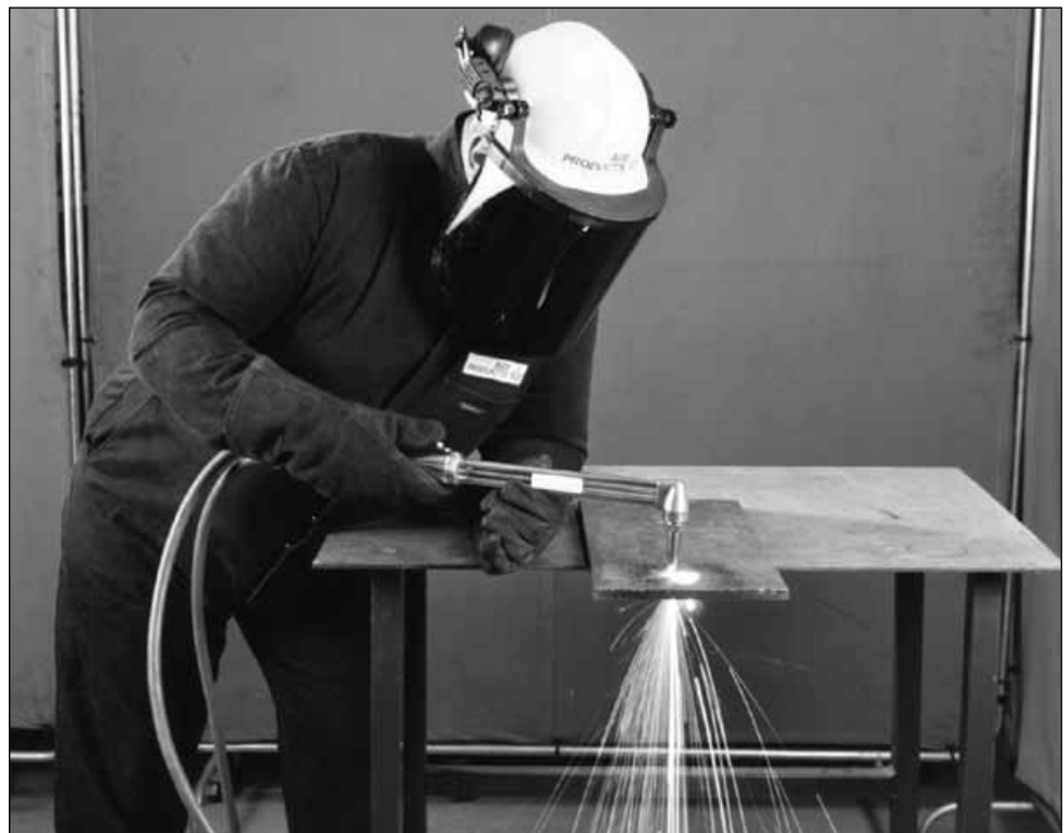
Figure 12 Flame cutting – use of protective equipment
