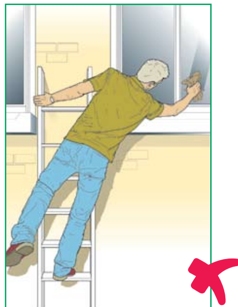
Figure 3b – This is an example of not using a ladder safely by reaching too far and not keeping three points of contact with the ladder
